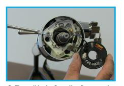
3. Then, slide the Canceling Cam over the column shaft and canceling cam spring. For proper operation of the canceling cam, align the canceling cam stem between the 10 and 11 o'clock position. (figure A)
