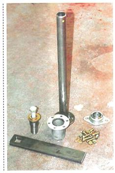
The conversion consists of an output shaft adapter that's splined to match either a reversed OE Corvair box or a Flaming River reversed box, an extension shaft that bolts to the adapter, a machined end piece for the shaft, and a straight cut Pitman arm. They also suggest the use of a shaft support (which they can supply as well) which will reduce the torsional twist on the steering box mounting bracket and output shaft.
