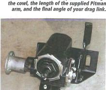
After two or three false starts I finally ended up sewing together a mounting bracket that located the box both in the correct position and solidly. Like I said, though the conversion components can be used to install a reversed Corvair box for cowl-steer in any situation, mounting the actual box will very from vehicle to vehicle.
