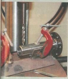
The next step is inserting the machined end into the extension tube. You'll want to pay attention to how you insert it as you'll want to make sure that the Pitman arm ends up hanging vertically when the extension shaft is bolted to the output shaft adapter, double check this before welding.
