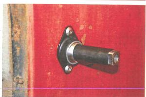
Once the welding was completed I carefully ground the welds smoothtaking my time so as not to damage the extension tube.
