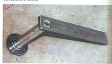
Before proceeding I took a few minutes to test fit the Pitman arm and then to prime and paint it and the shaft before reattaching it to the output shaft adapter.
