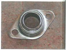
While placing my order for the kit with Gas Alley I opted to go with the suggested (but still optional) support bearing. The added support it offers will help keep any torsional effects to the steering box mounting to a minimum.
