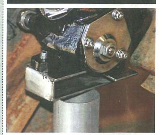
One thing that threw me off a bit is the fact that the mounting pad on a Corvair box is not horizontal—in other words, in order for the output shaft to be perfectly horizontal the mounting plate has to be tilted to the right by about 20 degrees or so (don't take my word though cuz I didn't write down my measurement).
