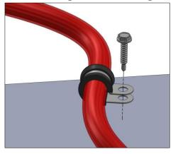
Use screws and insulated mounting clamps (not included) to secure cables to the vehicle.
