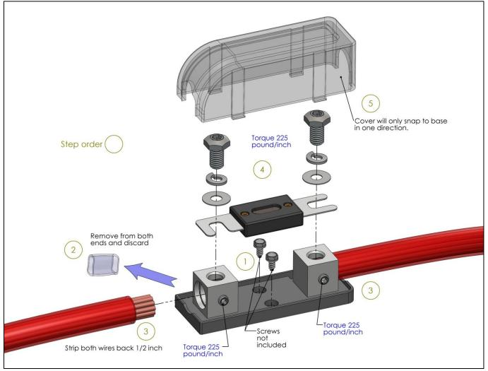
It is recommended a small amount of blue LOCTITE<sup>®</sup> be used on each ring terminal above screw. Do not get LOCTITE<sup>®</sup> on electrical connection surfaces because it is nonconductive.
