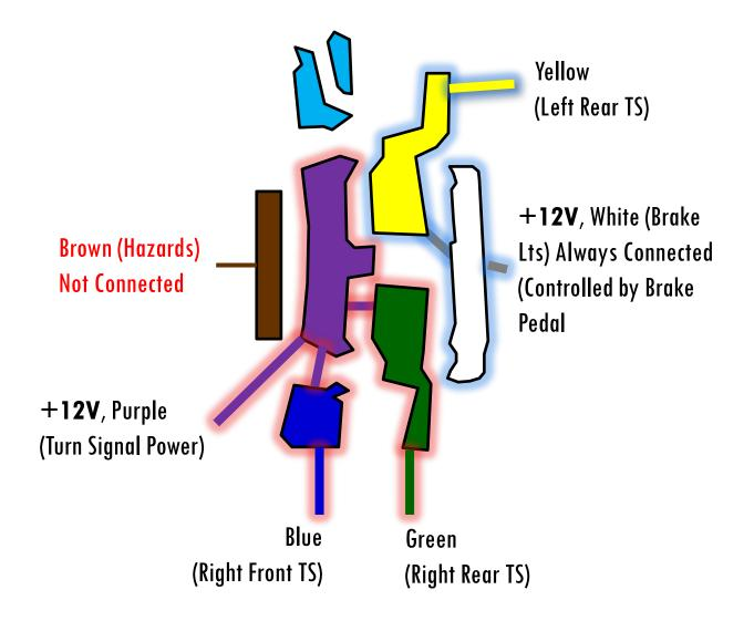
Turn signal power (Purple) connected to right side turn signals (Light Blue, Yellow). While Purple is connected to the right turn signals, these will flash on and off if a flasher is installed.
