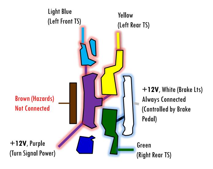
Turn signal power (Purple) connected to left side turn signals (Light Blue, Yellow). While Purple is connected to the left turn signals, these will flash on and off if a flasher is installed.
