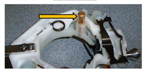
**IMPORTANT:** Spring-loaded horn contact connects to the underside of the cancelling cam. When connecting the cancelling cam to your horn button, please note the following:
