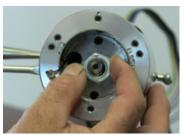
3. Place the steering wheel or adapter on the steering column shaft. Then place the retaining nut on the shaft and tighten, drawing down the wheel or adapter to the desired gap (we recommend approx. 1/16"). (DO NOT OVER-TORQUE)
