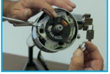
4. Place the final 3/16" aluminum spacer over the column shaft and down to the canceling cam.
