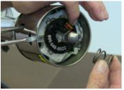
2. The compression spring is positioned over the column shaft on top of the canceling cam.
