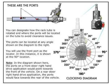
The ports can be positioned rotationally anywhere depending on where there is clearance. We need to know this information because once the tube and casting are pressed together and the drive pins are installed, the tube location is set.
