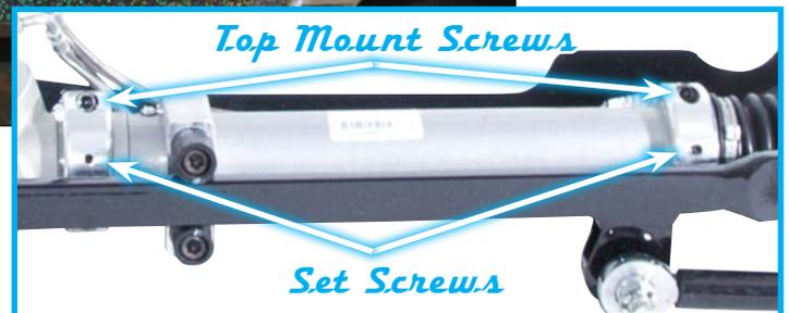
2) The Rack and Travel Bar Assembly comes mounted to the cradle, but can be adjusted to achieve different pinion angles by loosening the screws in the mounts and rotating the rack. Once it is positioned at the desired angle re-tighten all fasteners and make sure to tighten the set screw in the middle of the mount.
