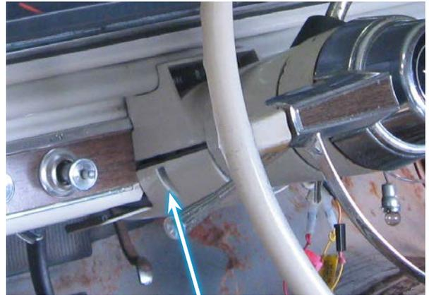
2) Remove the screws and dash bezel
