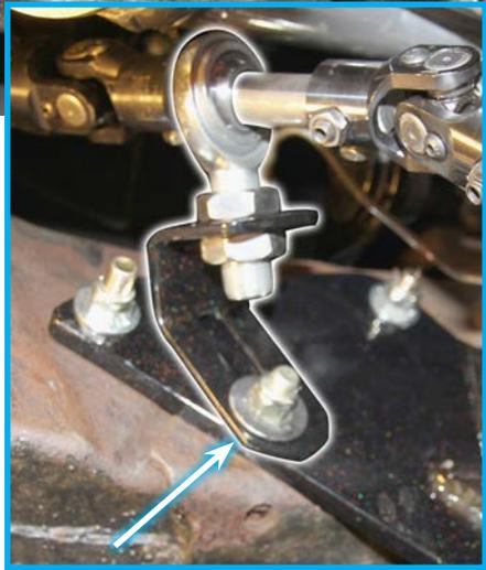
*Support Bearing and Bracket Mounting*
