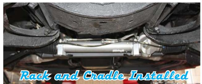
3) Install the OEM outer tie rod end into the Flaming River inner tie rod end on the new power rack. Note: If using the original parts some adjustment of the tie rod assembly may be required when connecting the to the spindle arm and the travel bar.
