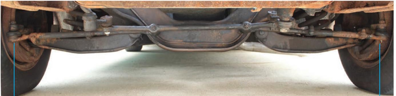
Before beginning you must first measure the width of your front end from LEFT outer tie rod end zerk to the RIGHT outer tie rod end zerk to determine the overall width of your front end. Write dimension here for further reference \_\_\_\_\_
