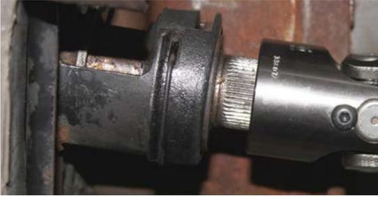
Note: Depending on u-joint alignment, It may be necessary to shorten the factory steering column by either trimming the the steering column shaft (63-66) or collapsing the column shaft (67-82) until the splines meet the end of the column tube. (example shown in picture to left).
