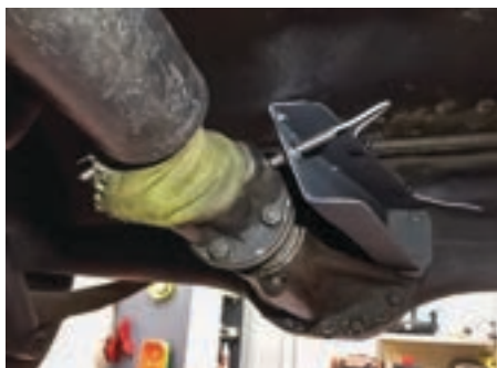
SENSOR MOUNTED ON PROPELLER SHAFT
