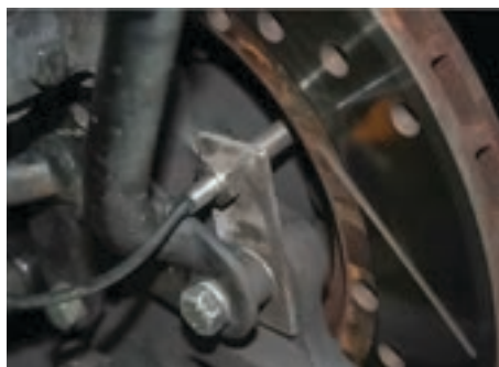
SENSOR MOUNTED ON BRAKE DISC
