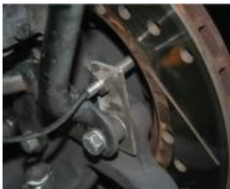
SENSOR MOUNTED ON BRAKE DISC
