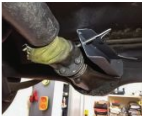
SENSOR MOUNTED ON PROPELLER SHAFT
