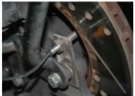
SENSOR MOUNTED ON BRAKE DISC
