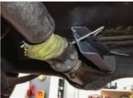
SENSOR MOUNTED ON PROPELLER SHAFT
