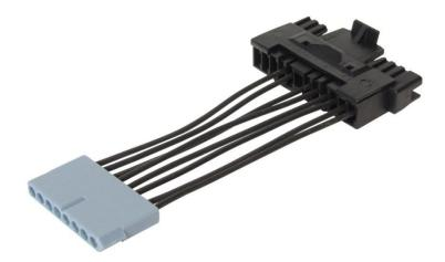
The Mopar Wiring Adapter (FR20118-6) unites the 4-1/4" female connector from your Flaming River column wiring harness with the stock 8-pin Mopar connector in your vehicle. This adapter is designed for Mopar vehicles from 1970 to 1974 that commonly use this style connector in turn signal switch wiring harnesses.
