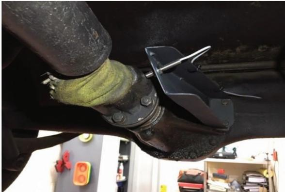
Sensor mounted on Propeller Shaft
