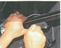
Flaming River gave a universal position column adapter to allow us to place the new steering column at any height we desired in the dash and firewall. We actually ended up moving the steering wheel a little closer to the driver's seat since the seating position has been pushed back farther from the dash.
