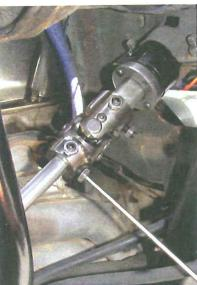
The Billet-Joints have allen set screws to hold the steering shaft to the column and steering box. It's recommended that you use a drill to make a dimple in the DD shaft where the allen screw goes.
