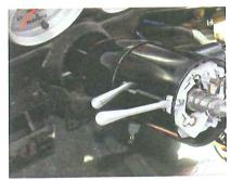
We also got the satin aluminum steering column dress-up kit that comes with a new tilt lever, signal lever, and hazard lights button. It gives an extra bit of appeal to the new column kit.
