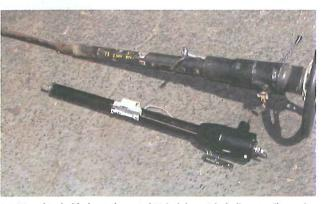
We ordered a black powdercoated 30-inch-long, 2-inch-diameter tilt steering column to replace our existing one. We could have got a polished stainless steel column, but we thought that might look a little too fancy in our old Chevy. We got the floor-shift style column since we had installed a B&M floor shifter some time ago and did not need a lever on the column, but we made sure to get a column with the ignition tumbler on the side since we did not have an ignition switch in the dash.
