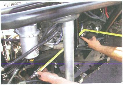
To cut the correct length steering shaft, we place the Billet-Joints on the steering box and the steering column and measured the length. This measurement does not have to be exact down to the millimeter because Flaming River uses a slip shaft for trucks.
