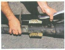
The connections were the same on the original GM column and the new Flaming River column (only rotated 180 degrees), so there was no need to cut wires and use adapters to get the signals and ignition to work.
