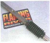
Flaming River's GM DD slip shaft comes in either 30- or 38-inch lengths. The slip part is covered by the protective collapsible boot, and there is a grease fitting to keep things moving smoothly. Yes, frames are not supposed to flex very much, but trust us, they do, and the smooth slip shaft feature is great for preventing the shaft from pulling off the steering box when collapsed and elongated during frame-twisting off-road situations.
