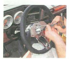
12 Gregory tightened the Cascade wheel onto our 6-bolt polished, tapered wheel adapter, and then reinstalled the horn button into the middle of the wheel
