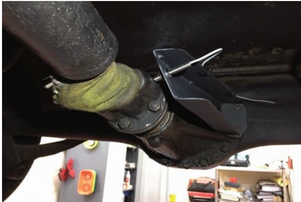
SENSOR MOUNTED ON PROPELLER SHAFT
